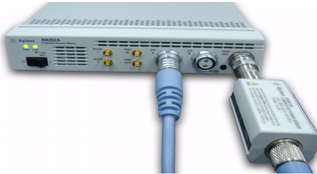
Figure 1-20 Connecting sensor to the PWR REF connector.
