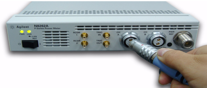
Figure 1-17 Connecting power sensor to CH A input connector.
