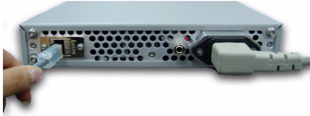
Figure 1-12 Connecting the LAN cable.
